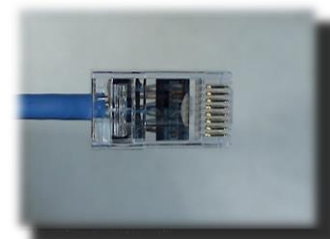
13. Insert prepped cable into plug housing. Bottom fully.
