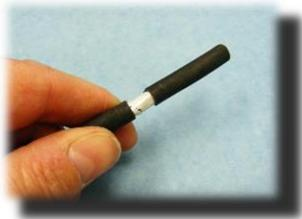
1. Strip outer jacket approximately 1 ½ inch. Install Boot over cable ends if boot is desired.
