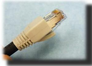
25. Install Optional Boot over back of Plug housing.
