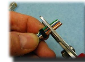
14. Cut Conductors leaving .140 to .160 inch from front of the Load Bar to the conductor tips.
