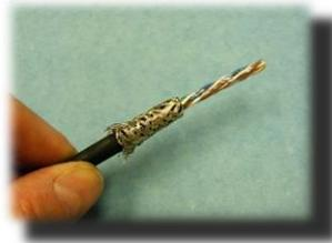
3. Fold back braid or foil then wrap drain wire around the outer jacket. (Foil can be removed if desired)
