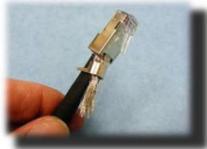
20. Bring braid or foil and drain wire to bottom for crimping as shown.
